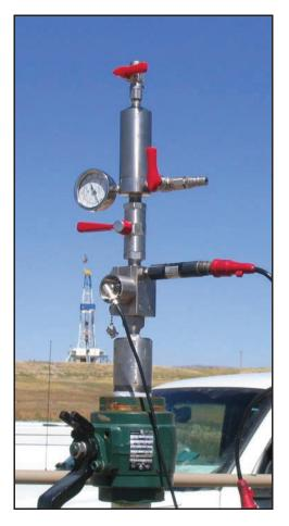
For best results, before attaching the gun to the wellhead, replace any needle valves with  $\frac{1}{2}$  inch ball valves in order to minimize energy loss through connection as shown below:
